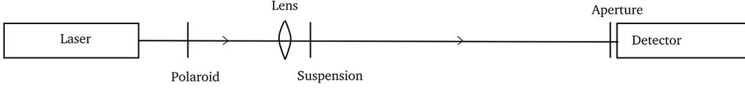
Figure 1: *Experimental setup. The laser and detector were aligned on an optical bench, with a Polaroid to control the intensity reaching the detector; a lens to focus the light onto the specimen - the suspension - and an aperture to ensure that we have a 'point' detector, so that the autocorrelation will be valid.*
