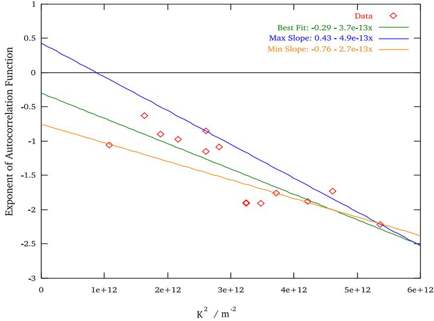
Figure 5: A plot of the exponent of the autocorrelation function against the square of the wave vector. The gradient gives us the diffusion constant, and in turn Boltzmann's constant.
