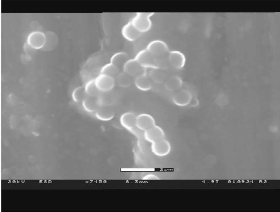
Figure 4: *Environmental Scanning Electron Micrograph of the latex spheres that we used in suspension.*
