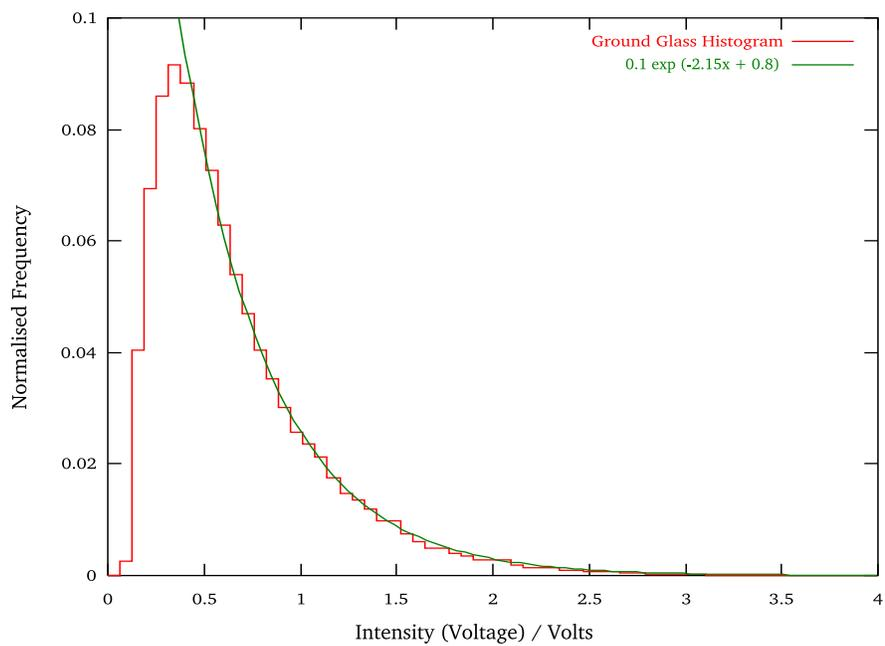
Figure 2: Histogram of  $I(t)$ , which shows the probability  $p(I)$  of finding an intensity  $I$  between  $I$  and  $I + dI$ . This shows that scattered laser light is indeed Gaussian, as it behaves as  $p(I) \propto \exp(-I/I_0)$ . The exponential decay does not quite start at zero intensity because of background ambient light.
