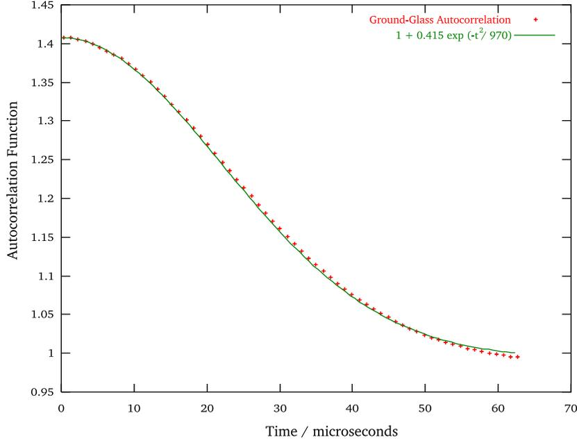
Figure 3: Autocorrelation function for a rotating ground glass slide, moving at 2 r.p.m. The solid green line indicates a Gaussian fit to the data.
