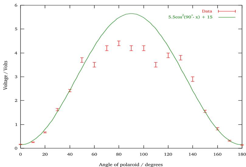
Figure 6: A plot of the voltage output of the light detector with the angle of the Polaroid. The solid line indicates a Malus' Law ( $\cos^2 \theta$ ) fit to the data. This fit fails at high voltage as the detector stops being linear, and eventually saturates.
