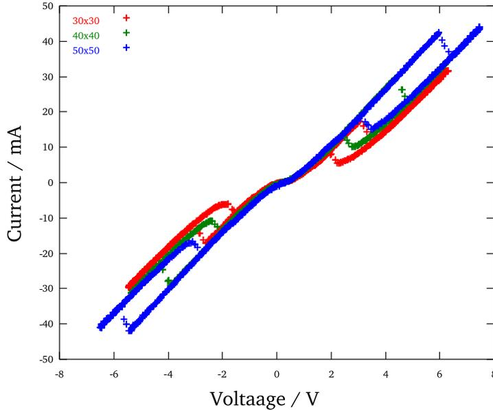
Figure 8: *Hysteresis in resonant tunnelling diodes. The hysteresis is more noticeable they larger the area of the device.*
