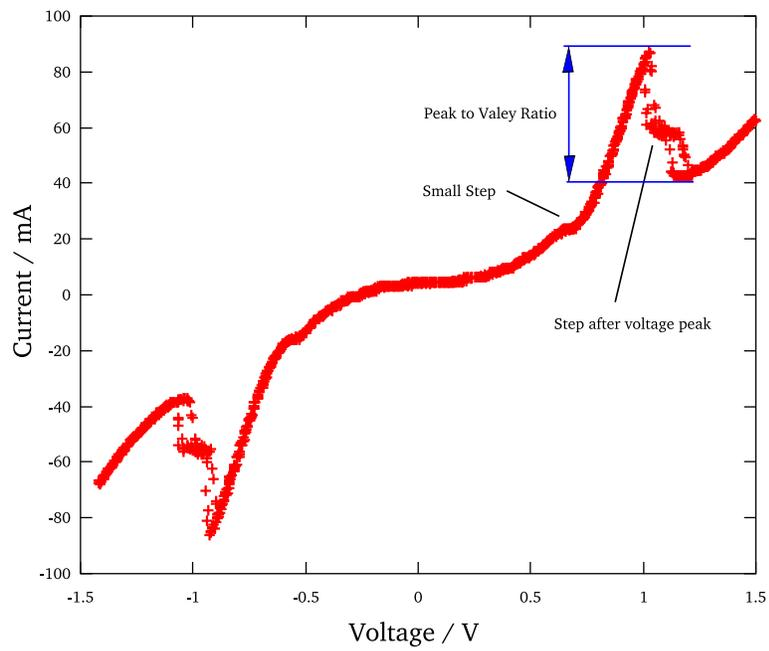
Figure 9: A current-voltage plot for a resonant tunnelling diode. The device used has a well width of 6nm, the surround barriers are 3nm wide, and the area of the layers is  $20 \times 20$  micron.
