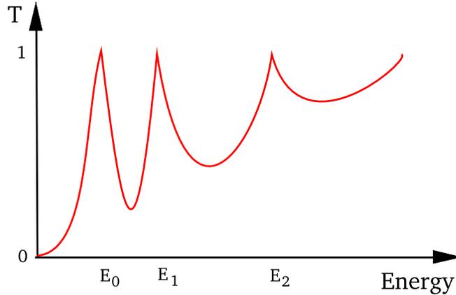
Figure 7: *The transmission coefficient as a function of energy. The resonant peaks correspond to allowed well energy levels. The general increase in  $T$  with energy (temperature) is due to greater number of phonons for electrons to scatter off, to enter the permitted energy levels.*
