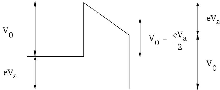
Figure 2: With a voltage across it, the barrier behaves as shown, and now has an effective height of  $V_0 - \frac{eV_a}{2}$
