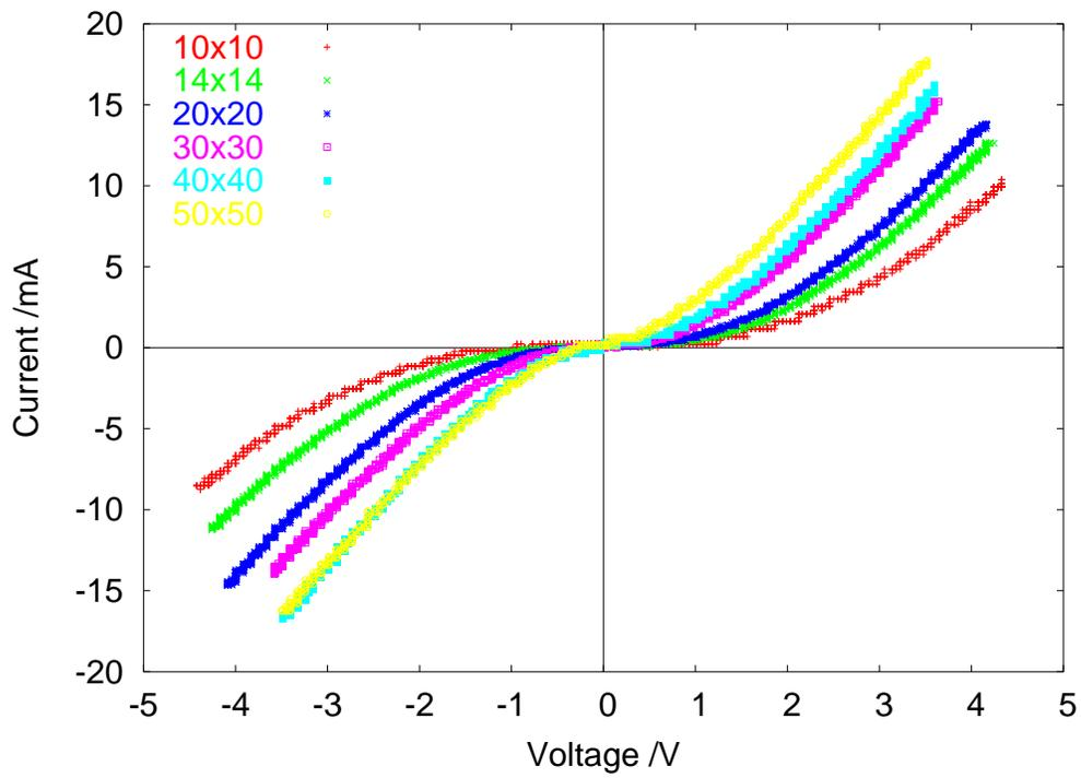
Figure 5: *The I-V curves of the variously sized area wafers of the wide single barrier*
