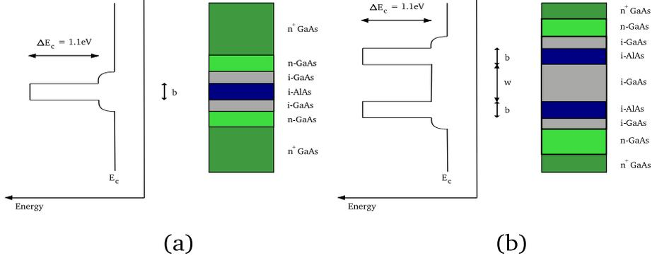
Figure 1: *Quantum barriers and wells produced by layering III-V semiconductors with different conduction band energies. The width of the single barrier is either 2nm or 3nm depending on devices. The width of the wells is either 6nm or 9nm. The doped layers surrounding wells allow electrons to flow to the wells. These layers are then connected by gold wire to soldered contacts with copper wire to our measuring equipment.*
