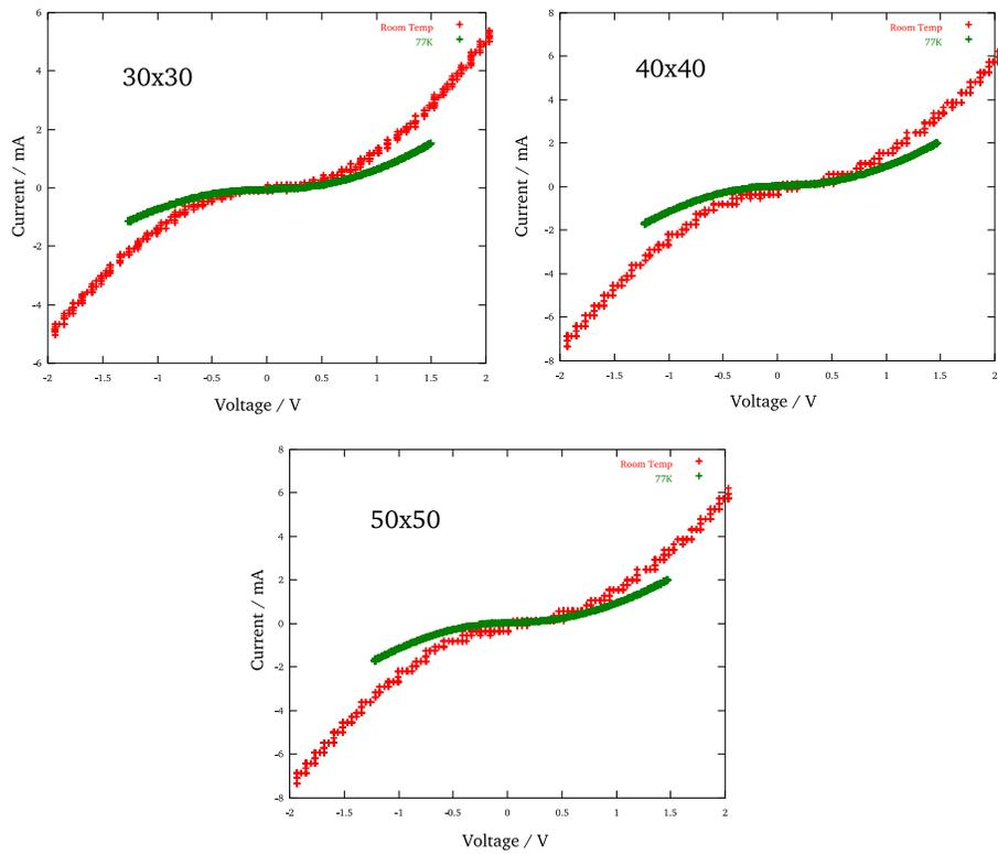
Figure 6: A graph showing the effects of temperature on the I-V characteristics of a single barrier. The red curves represent room temperature, and the green ones 77K.
