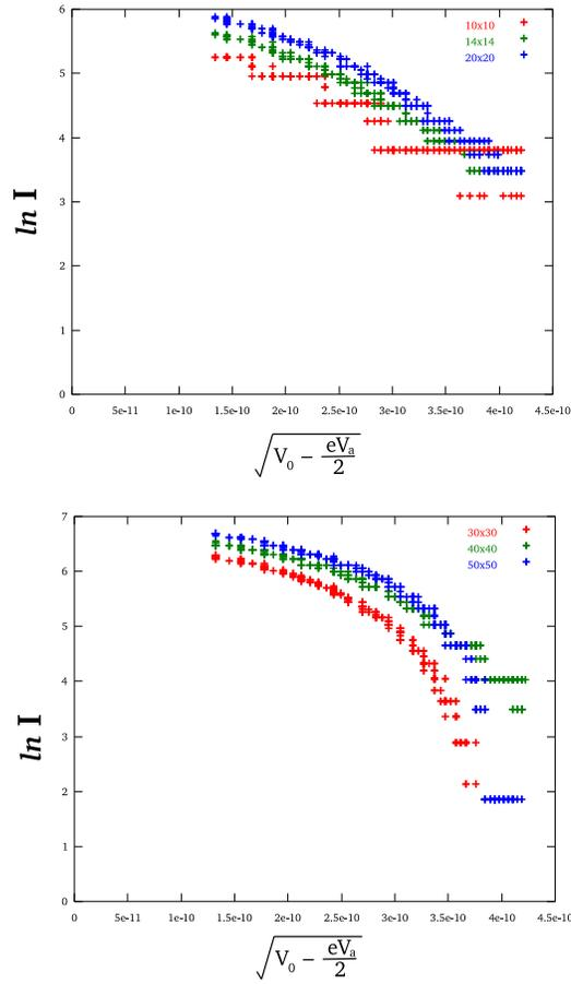
Figure 3: The gradient of lower right part of this slope gives an estimate of the barrier width. This is the 3nm barrier, and the key shows the areas of the semiconductor layers, in microns. The horizontal areas arise due the lack of precision in the voltmeter in measuring very small currents.
